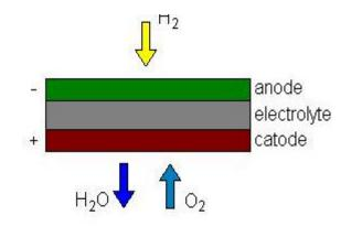
Figure 1. - Schematic of one type of fuel cell.
